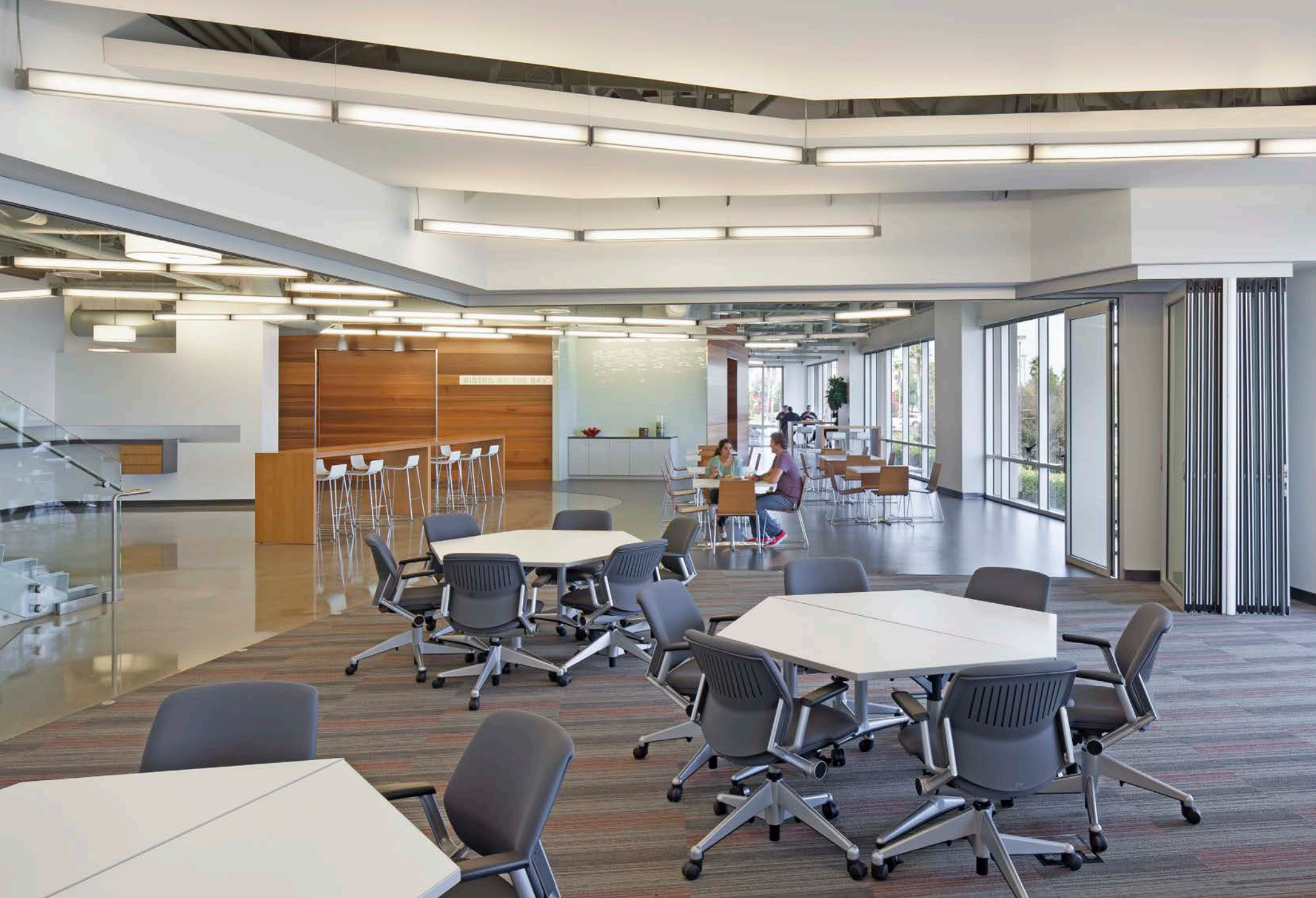
Actelion, San Francisco CA NanaWall HSW60 , aluminum framed single track sliding system, panels stack away from opening, no floor track, open corner configuration with swing door Architect: Rapt Studio
