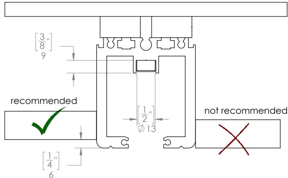
IF YOU WANT TO RECESS THE HEAD TRACK INTO THE CEILING, WE RECOMMEND TO LEAVE 1/4" (6MM) VISIBLE TO AVOID SCRUB MARKS FROM THE TOP BRUSH SEALS IN THE AREA OF THE SWING PANEL, STACKING BAYS AND 90° CORNER TURNS.
