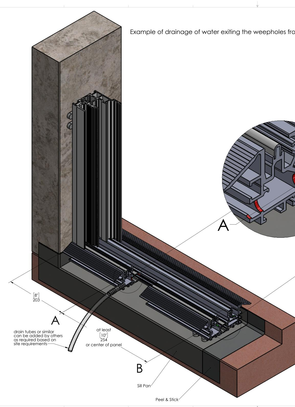
Example of drainage of water exiting the weepholes from NanaWall low profile saddle sill ("LPSS") for the Generation 4 systems
