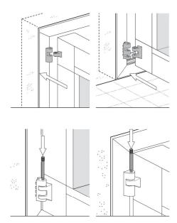
Do not force any hinge pins – check for obstructions in the hinge barrels. Tap the hinge pins in so the knurling on the end of the pin is all the way in, but let the hinged dome protude slightly.
