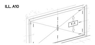
Check the fastened sill to make sure that it is level, and not tilted or twisted. Loosen fasteners and adjust the height of the shim stacks until the sill is at the correct elevation, and perfectly level without any tilt or twist. Make sure that all holes drilled through the sill are properly sealed with exterior grade polyurethane sealant underneath and around the screws. All weep holes in the sill, if present, are not to be obstructed.
