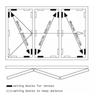
Follow all proper applicable glass installation and glazing techniques as recommended in the Flat Glass Marketing Association (FGMA) "Glazing Manual" and "Sealant Manual". Always use suction cups to shift glass within an opening. It would be best to install the glass on the panels before they are installed in the opening. Panels can be laid flat on sawhorses. If the panels are already installed, they can still be glazed.
