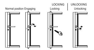
Disengaging locking points (Note that this is not one motion operation. Key or thumb turn must be unlocked first.)
