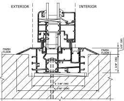
LOW PROFILE SADDLE SILL – OPTION 1 (Weep holes by others necessary for water rating as lab tested)
