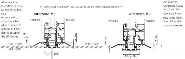
Note: If the finish floor is at a different level than shown, appropriate landing on both sides of the threshold with ADA-compliant slope must be constructed.
